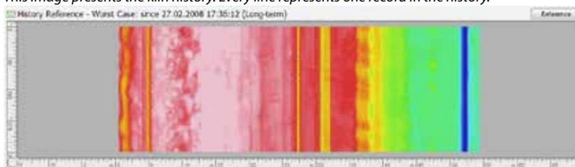
This "worst case image" is a thermal image composed from many thermal images taken from the kiln history. Every point shows the maximum temperature measured at this point since the indicated time.
