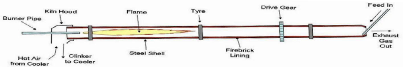
Schematic representation of a rotary kiln
