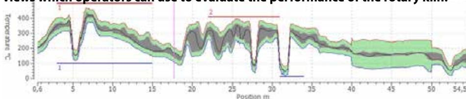
Permissible temperature envelope profile with the possibility to define individual limits for different kiln zones
