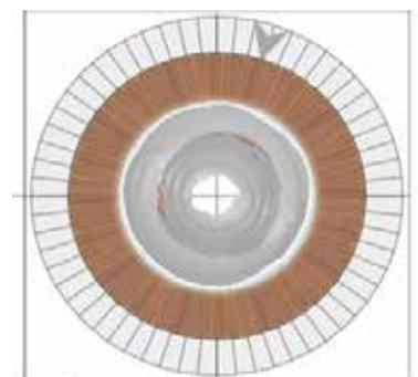
*The kiln end-view is a special case of the Kiln Section 3D view.*
